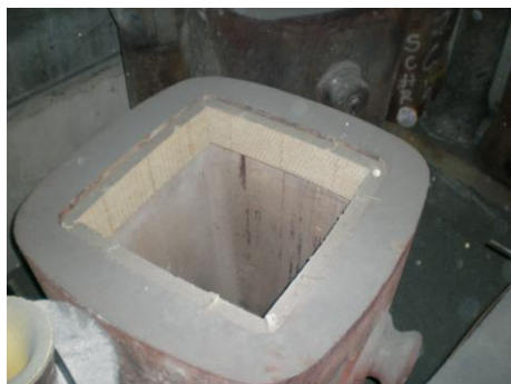
Figure 2: 4.5 ton mould with insert-feeder
